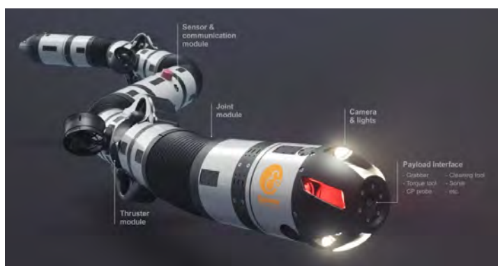
Figure 1: "Aluma" – "Snake Robot" capable of repairing pipes on the ocean floor 4
